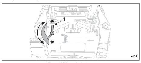
Figure 3-33 Creep Control Lever
